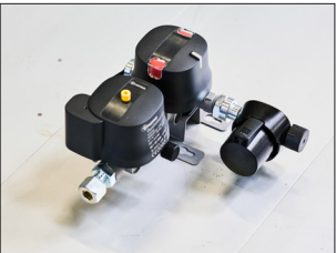
DuoControl – automatic gas changeover with crash sensor that cuts the gas supply on impact at 3.5 G. Approved for gas operation while driving across Europe.
