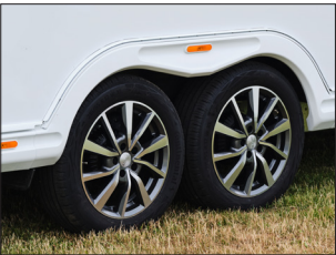
Tandem axle is standard in the European markets for specific models
