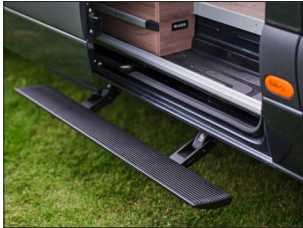
Electric step (four-wheel drive only) • driver/passenger door • large sliding door • at all three door openings
