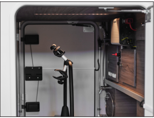
KABE's practical bike rack – carry and store your bikes in the motorhome's garage. The rack pulls out for better ergonomics and has a smart extra module that lets you turn the handlebars to make the most of the available space (not for Novum LXL and x810 LXL/LT).
