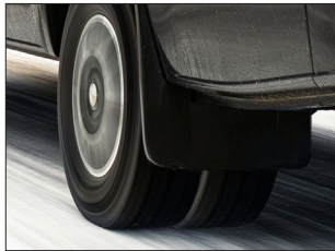
Twin wheels 4 x 2 and 4 x 4 5 tonnes, approx. 850 kg extra payload, train weight 7 tonnes
