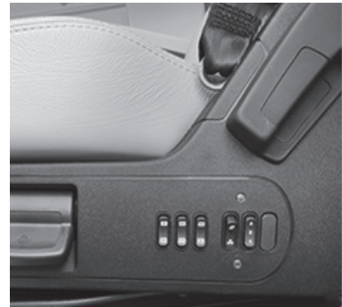
Buttons on the outside of each seat control their heating and cooling.
