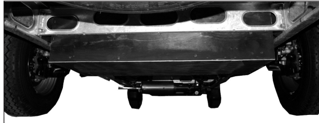
The grey water tank is mounted close to the motorhome's rear axle.
