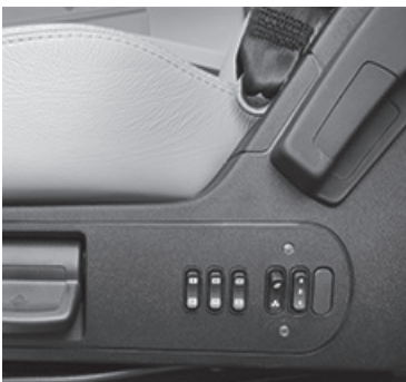
Buttons on the outside of each seat control their heating and cooling.
